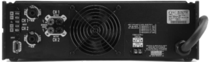
The amplifier shall employ forced-air cooling with a variable speed fan for minimum acoustic noise. Air flow shall be from rear to front to avoid temperature rise inside the rack. Rack mounting shall be possible without clearance between amplifiers for ventilation. The amplifier shall be capable of continuous operation at 1/3 power, into four-ohm loads, for ambient temperatures up to 104° F (40° C).
